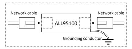
Note: Due to the bi-directional structure of the ALL95100 Surge arresters the input and output side is arbitrary exchangeable.
