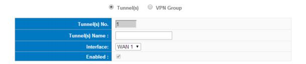
**Tunnel No.:** Set the embedded VPN feature, please select the Tunnel
