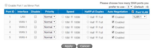
Mirror Port:Users can configure LAN 1 as mirror port by choosing "Enable Port 1 as Mirror Port". All the traffic from LAN to WAN will be copied to mirror port. Administrator can control or filter the traffic through mirror port. Once this function is enabled, LAN 1 will be shown as Mirror Port in Physical Port Status, Home page.
