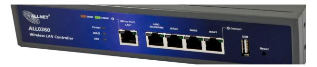
**WAN** connection: A WAN port can be connected with xDSL Modem, Fiber Modem, Switching Hub, or through an external router to connect to the Internet.
