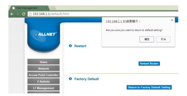
It's recommended to save the current configuration before upgrading firmware. After firmware upgraded, import the configuration file after returning to factory default to ensure system stable. (Please refer to 12.3)
