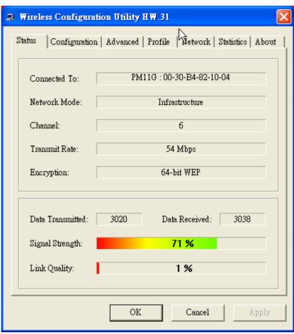
There are two dialog boxes showing the data transmitted and the data received. The two signal lines show the Signal Strength and the Link Quality of the device.
