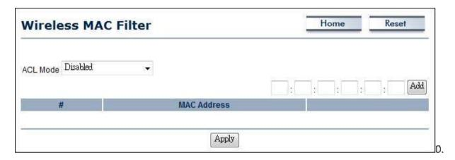
Wireless MAC Filters are used to allow or deny network access to wireless clients according to their MAC addresses. You can manually add a MAC address to restrict the permission to access ALL0258N. The default setting is Disable Wireless MAC Filters.
