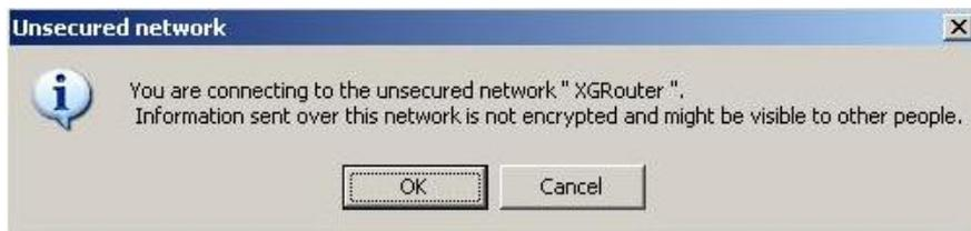
5. Click 'OK', and fill your information in the 'Wireless network properties', or just click 'OK'. If the wireless access point has enabled encryption, you will have to input the WEP key or WPA preshared key in the form.
