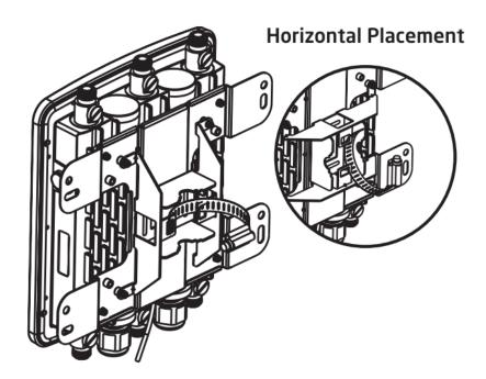
**D)** Determine where the device is to be mounted. Lock and tighten to secure the mast holder to the mast.
