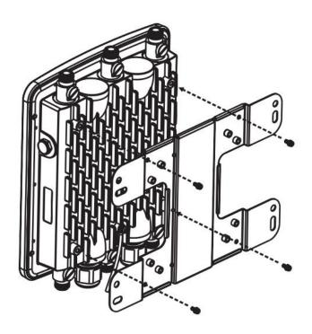
**B)** Determine which assembly is to be mounted. Tighten the four round head screws to secure the post holder to the mounting base.
