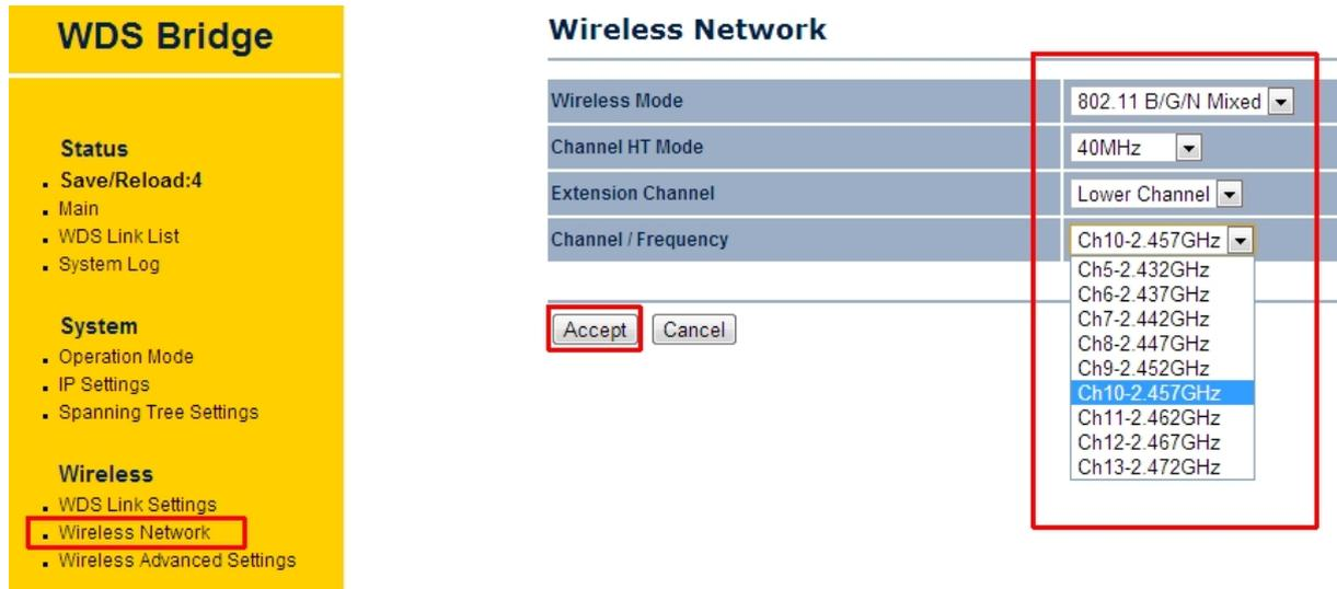
The screenshot shows the configuration interface for a WDS Bridge. On the left is a yellow sidebar with a menu. The 'Wireless' section is expanded, and 'Wireless Network' is selected. The main area shows the 'Wireless Network' configuration page. The 'Channel / Frequency' dropdown menu is open, showing a list of channels. 'Ch10-2.457GHz' is selected and highlighted in blue. The 'Accept' button is also highlighted with a red box.
