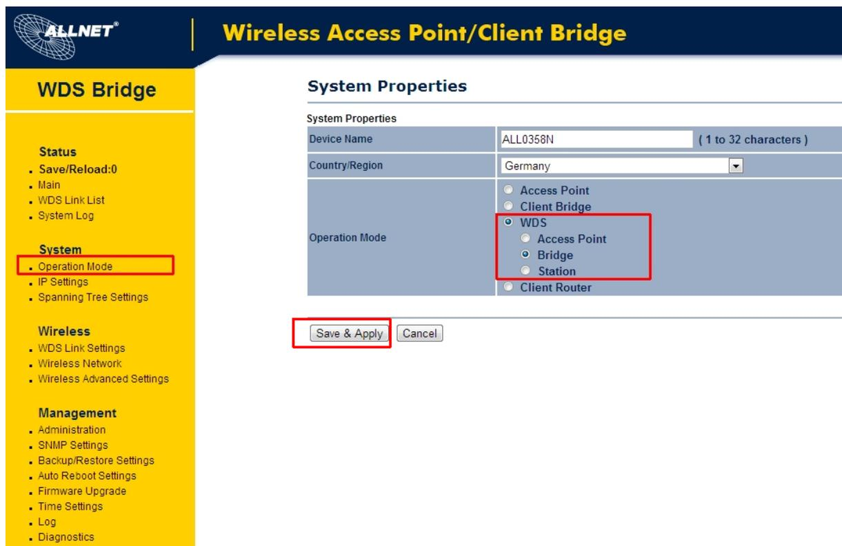
The screenshot displays the ALLNET web interface for configuring a Wireless Access Point/Client Bridge. The left sidebar shows the navigation menu with 'System' > 'Operation Mode' highlighted. The main content area is titled 'System Properties' and contains the following fields:
