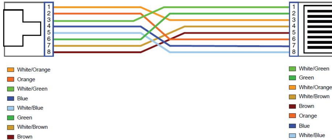
Figure C-3 Pin Assignments and Wiring for an RJ-45 Crossover Cable
