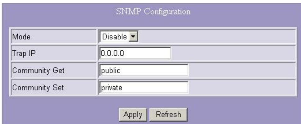
The image shows a web-based configuration interface for SNMP. The title is "SNMP Configuration". It contains four rows of configuration fields:
