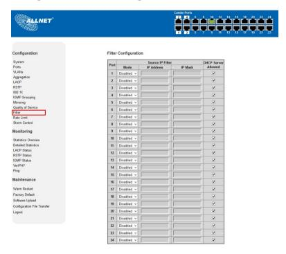
Select the "Port no." which you want to configure the mode to enable/disable filtering IP address.
