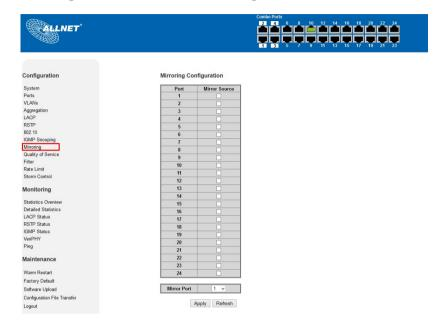
Port Mirroring is for mirror the traffic from Source port to Destination port.
