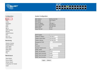
It shows system status, such as: MAC address, system firmware version and so on.
