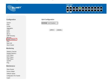
You can enable or disable QoS by clicking the checking box. If you enable QoS, you can select the class of service for each port.
