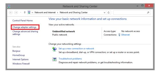
A **Network Connections** window will pop up, **showing** all the network 2. connections available on your PC. Please double-click on the network connection you are using to connect the device.
