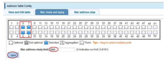
2) will be dropped or learn the Mac address of the port equipment after 2 minutes disappear automatically from the Mac address table
