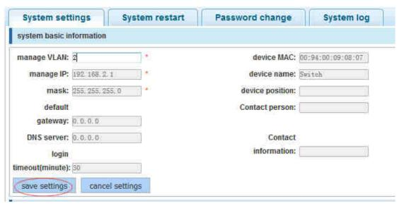
2) insert the PC interface 9 or 10 ports, set up the management IP for 192.168.2.12, device name is yoyo, timeout for 20 minutes
