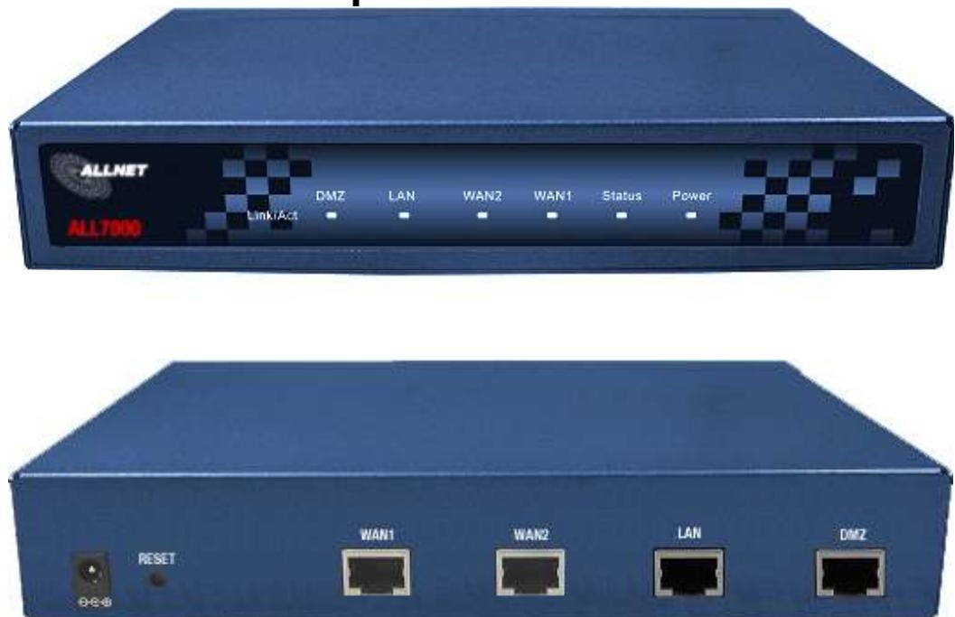
**WAN 1 Port:** Use this port to connect to the external router, DSL modem, or Cable modem.
