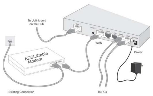
**Figure 4: Installation Diagram**
