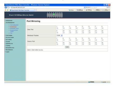
Port Mirroring is used to mirror traffic, RX, TX or TX&RX, from Source port to Destination port for analysis.
