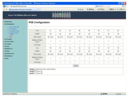
Remote access and monitor the attached PD (Powered Device) status by using Enable/Disable function.
