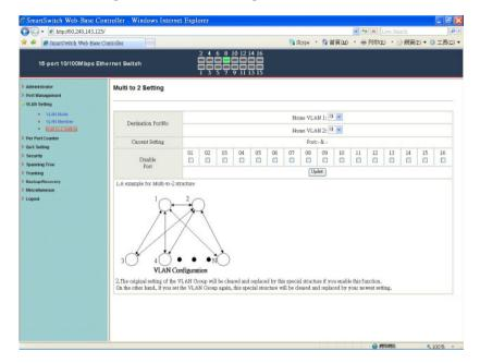
This is a special design for easily setting the switch VLAN into "VLAN Per Port".
