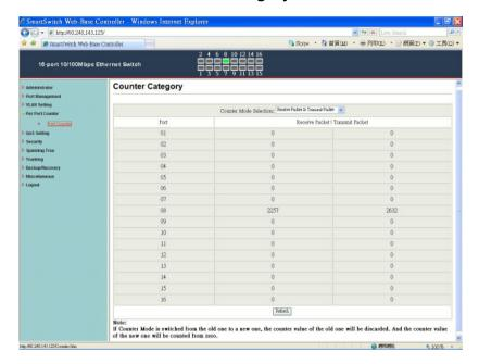
You can read the transmitting and receiving packet of the connecting port.
