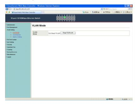
There are two VLAN modes: Port Based VLAN and Tagged VLAN.
