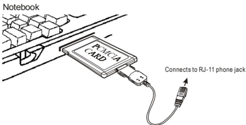
3. Connect the other end of the PC Card cable to the telephone line outlet.
