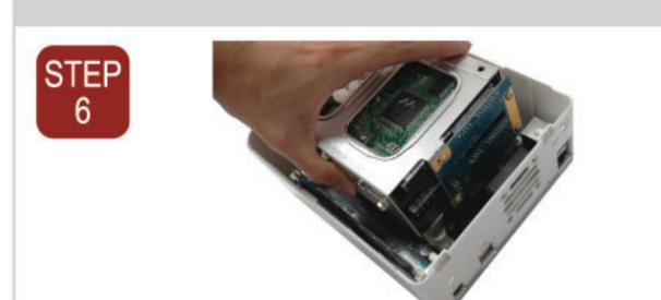
After making sure the tray is in place and the connectors are aligned, secure the hard disk tray with screws.
