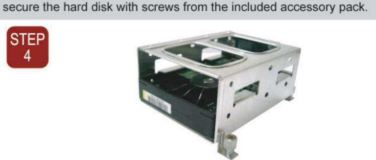
If you are installing two hard disks, please insert the second hard disk at the bottom of the tray and secure it with screws from the included accessory pack.
