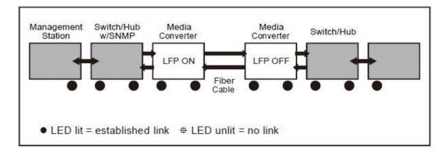
If one of the optical conductors is down (as shown in the diagram box below), the converter with LLR function will return a no-link condition to its link partner. With LLCF function also enabled, the no-link condition is carried forward to the switch/ hub where a trap is generated to the management station, and the administrator can then determine the source of the loss.
