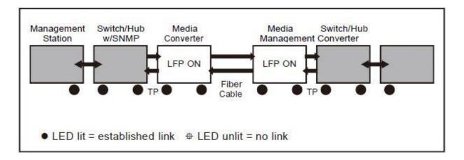
If the connection breaks, ALL-MC202P-SFP1-PoE that link loss forward to the Switch / Hub that generates a trap to the management station. The administrator can then determine the source of the problem.
