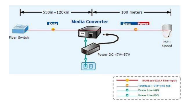
For the places where are hard to find the power inlet, the ALL-MC202P-SFP1-PoE provide the easiest way to power your Ethernet devices such as IEEE 802.3at / 802.3af Power over Ethernet Splitter with Internet Camera or PoE Wireless Access Point installed in the wild rang place.
