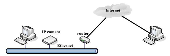
(2). IP camera connect to the Internet directly, if it's a fixed IP which provided by ISP, just input it. If it's a floating IP, then input the account and password which provided by ISP to dial-up connection.
