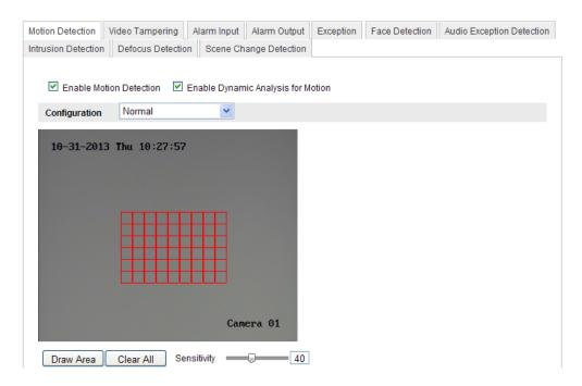
Figure 6-37 Enable Motion Detection
