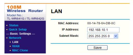
Figure A.2.2 Set the LAN parameters
