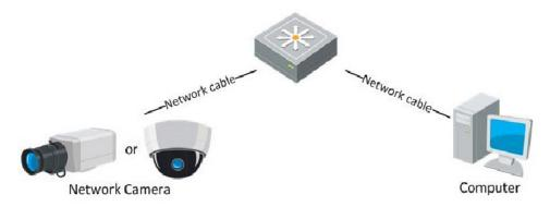
Figure 2-2 Connecting via a Switch or a Router
