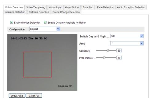
Figure 6-41 Expert Mode of Motion Detection
