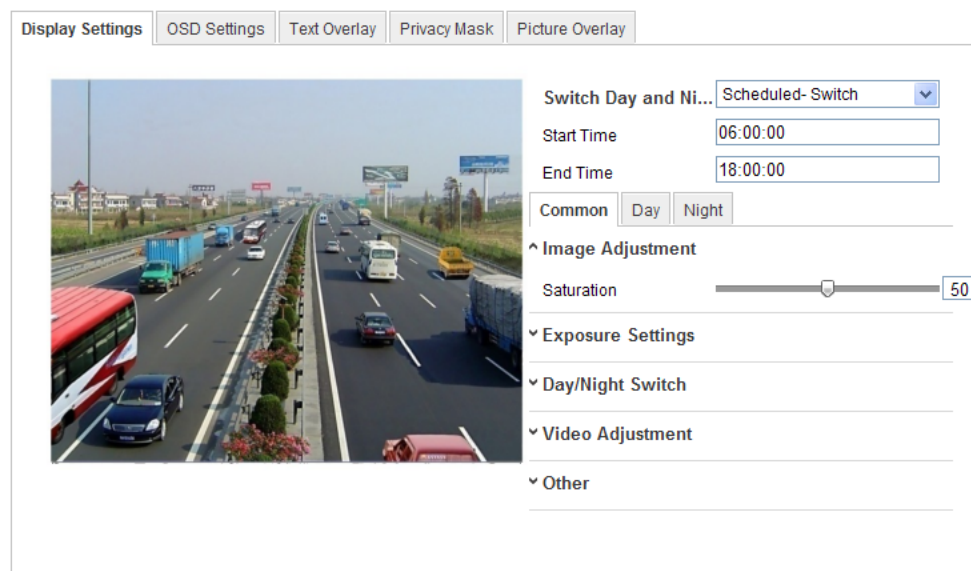
Figure 6-31 Day/Night Scheduled-Switch Configuration Interface
