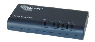
This very compact switch is especially suited for using in SoHo environment. The five RJ45 network ports automatically detect the transmission rate of the connected devices (10 or 100Mbit/s). By the full-and half-duplex operation, a maximum of 200 Mbit/s per port available.
