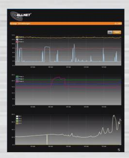
The live chart of the device shows you the actual power consumption of your house installation. You can compare different power phases directly to each other.
