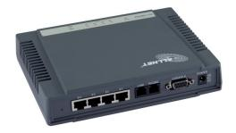
Via the **ALLNET ALL126AM2 VDSL master modem** in conjunction with the **ALLNET ALL126AS2 VDSL slave modem** dedicated lines can be realized by a simple 2-wire copper cable with a length of up to 2.5 kilometers. For short distances bandwidths of up to 100 Mbit/s are possible.
