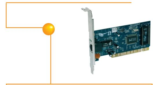
The ALL0119 is a 32-bit 10/100Base-TX Fast Ethernet PCI network interface card. It delivers the reliable quality, superior performance and ease of installation. This card features N-Way auto-negotiation, for automatic selection of the network speed and full/half duplex mode with the partner. Moreover, the Wake-On-LAN function is supported for network management.
