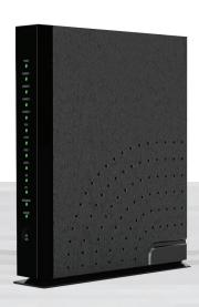
The ALLNET wireless AC access point works at the 2,4 or 5 GHz frequency range and achieves data transfer rates up to 900 MBit. Which means that it can fully utilize the speed advantage of the current technology.
