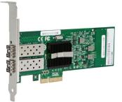
The ALLNET ALL0130-2SFP Multi-Port Server Adapter is PCIe GbE network adapters. Built with the Intel 82576 Gigabit Ethernet Controller, these new adapters showcase the next evolution in GbE networking features for the enterprise network and data center. These features include support for multi-core processors and optimization for server virtualization.
